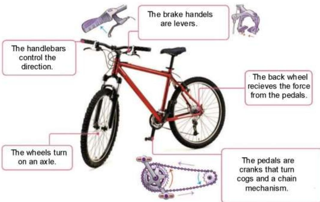
28<sup>th</sup> What is the name of the simple machines which made a complex machine?
